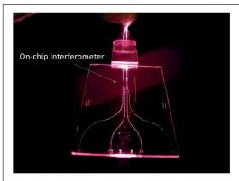
Photonic boards based on planar waveguides can also be employed for advanced functionalities such as on-chip interferometry, which helps to drastically reduce the footprint of industrial or environmental sensor systems [1].
