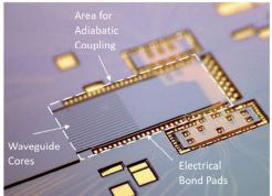
When manufactured on top of a PCB substrate, polymer waveguides can be used for simultaneous electrical- and optical coupling to a PIC (e.g. SiPh, InP) [2].
