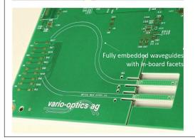
Fully embedding polymer waveguides into complex PCBs enables true on-board optical systems [3,4]. By bringing the optical signal closer to the chip, such systems provide tremendous advantages in terms of low power consumption and allow to reduce the amount of disturbing glass fibers inside a package [5].
