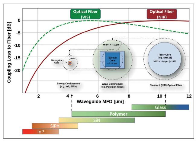
> The coupling loss to standard optical fibers as a function of waveguide modefield diameter (MFD). Several PIC platforms have emerged over the last decade, from strongly confined chips with large coupling loss to weaker confined platforms such as polymer or glass, with good overlap to optical fiber modefields.
