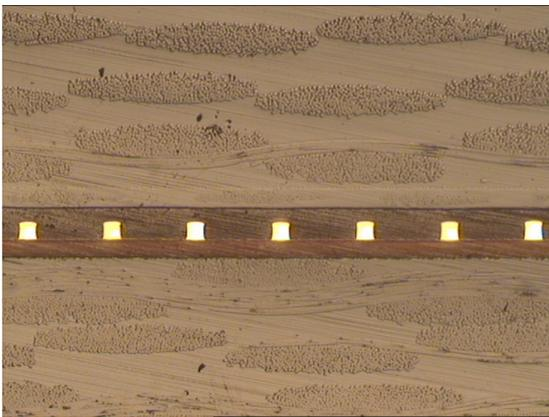
*Fig. 1: Optical inner layer with seven planar waveguides*
