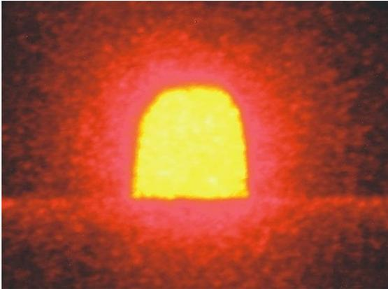
Fig. 3: Cross section of a planar waveguide
