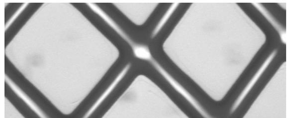
*Fig. 2: Crossing waveguides*
