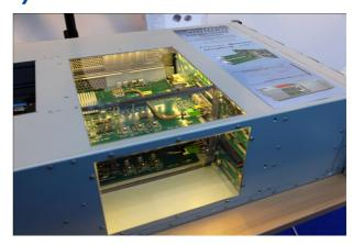
The system consists of a midplanedaughter card system. Finisar provided their high-speed optical engines which support 12 x 12 Gbit/s bidirectional bandwidth (12 x 28 Gbit/s are waiting in the communication wings). The based on 2 x 12 waveguides with a dimension of 50 µm. They are plugged together **Huber + Suhner's** via optical backplane connectors. presentation triagered a hiah level of interest from those **Booth B1.634**
