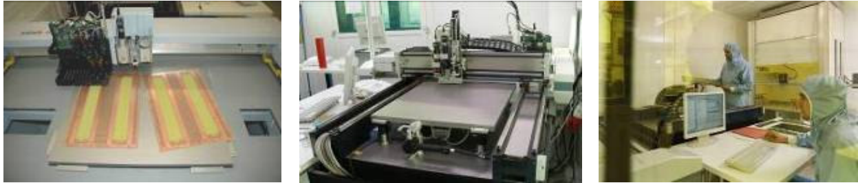
Fig. 5 EOCB manufacturing infrastructure: Polymer Coating, Laser Direct Imaging and Clean room
